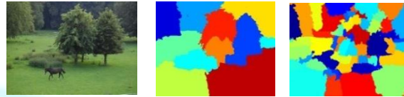
Fig. 1. Segmentation of a natural scene in (a) using the Normalized Cut algorithm for two different values of its input parameter (the expected number of regions) 10 and 60 are shown in (b) and (c), respectively.
